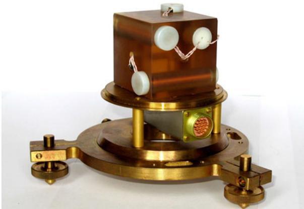
**Fig. 6** Three-component FGS with glass–ceramic housing
