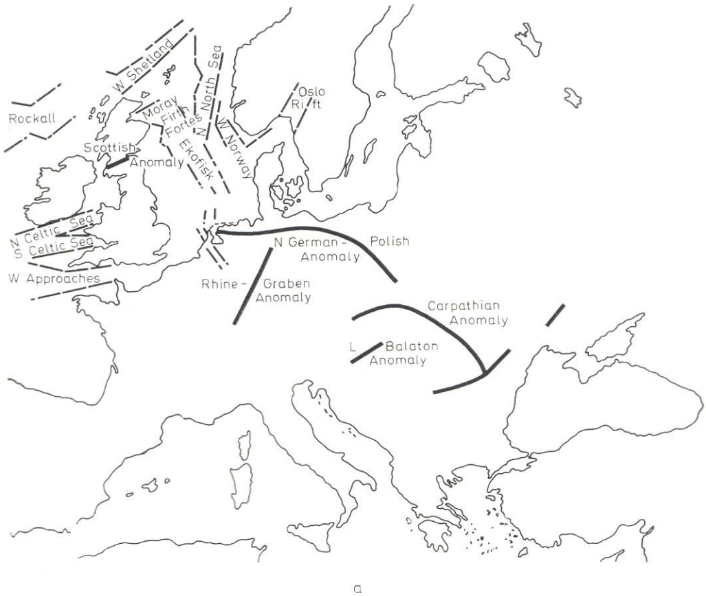
Fig. 12a. A map of Europe showing (i) the location of the conductivity anomalies indicated by available Weise vectors (after RITTER [70]) and (ii) a schematic representation of the position of the rifts in the North Sea as suggested by seismic investigations
