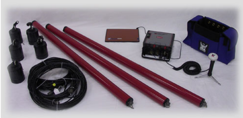
Figure 4.3.: Phoenix V5-2000 MT system. From left to right: non-polarizing lead, lead-chloride (Pb - PbCl) electrodes, induction coil cables, MTC-50 induction coils, battery, recording unit, case for the unit, and GPS antenna. Photo courtesy Phoenix Geophysics.
