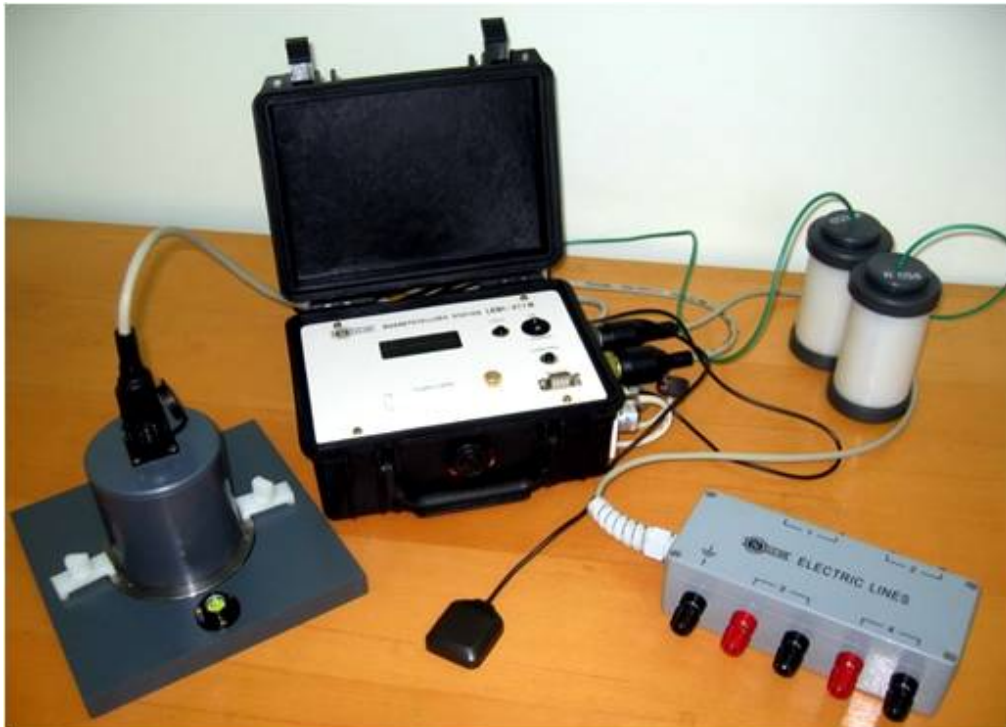
Figure 4.5.: The Long-period Magnetotelluric Instrument (LMTI) LEMI-417M. From left to right: fluxgate magnetometer with 10 m cable and installation platform, electronic unit (black box), the lead-free non-polarizing copper, copper-sulphide ( \text{Cu} - \text{CuSO}_4 ) electrodes, electric lines terminal, and GPS antenna.
