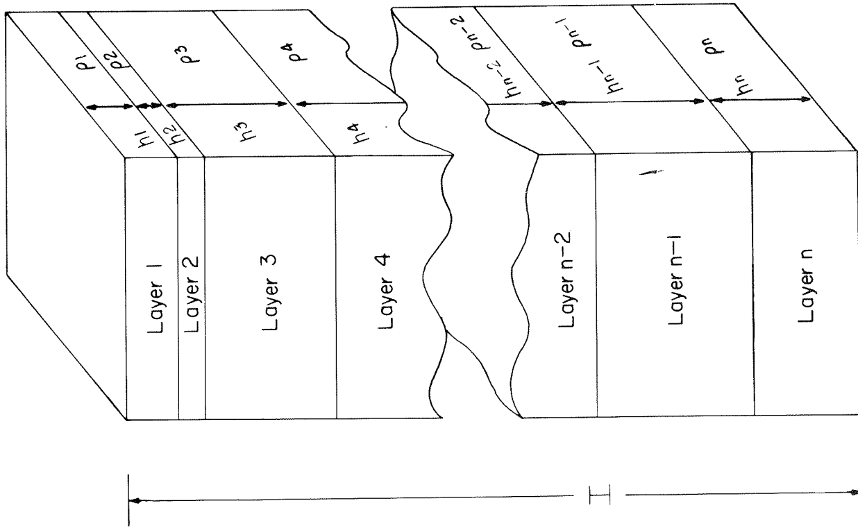
FIGURE 3.—Column from a layered sequence of rocks, used in defining average longitudinal resistivity, average transverse resistivity and anisotropy arising from layering.
