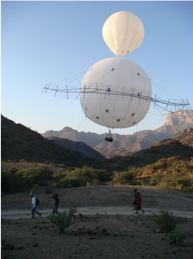
Fig. 1 Balloon-mounted airborne system. The transmitter is a 10-m-diameter wire loop suspended around a 5-diameter helium balloon. There is a second 2-m helium balloon added for additional buoyancy. Figure courtesy of Edgar Stettler and Thani Dubai Mining LLC
