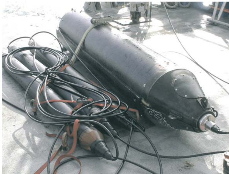
Figure 15. Photo image of the magnetic dipole–dipole system. The system forms a 50 m long array on the seafloor and is dragged along the seafloor at speeds of 1–2 knots. It consists of a transmitter and three receivers at distances 4, 13, and 40 m from the transmitter, capable to investigate the shallow sediment structure to 20 m below the sea floor.
