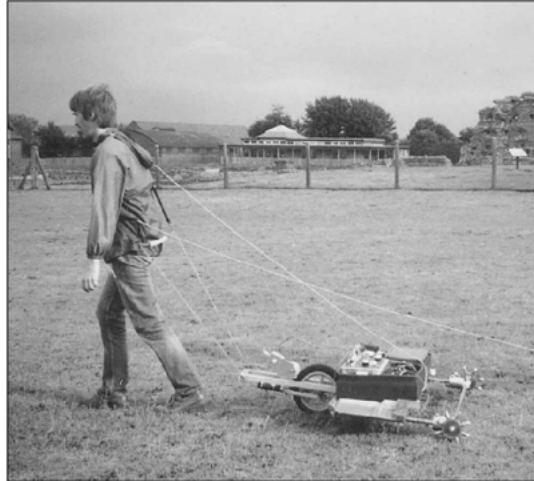
(a) mobile, pole-pole array system
