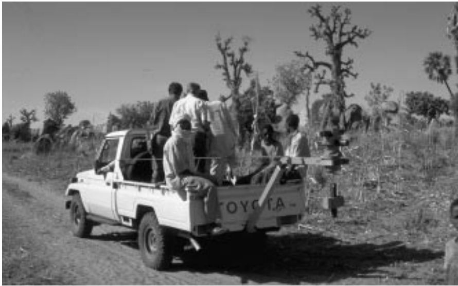
Figure 14. Car with automatically oriented antenna fixed behind for car-borne VLF measurements (Stiefelhagen, 1998).
