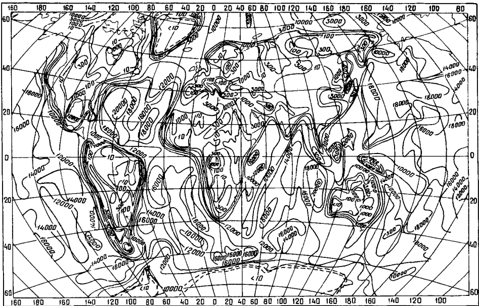
Fig. 4. Map of total conductivity of water shell and the Earth's sedimentary cover.
