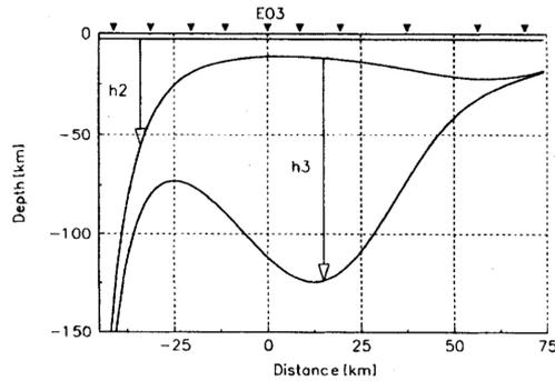
Fig. 2. Final 4-layer 2-D model with station sites (arrows). Thicknesses  $h_2$  and  $h_3$  are computed with the final polynomials. Resistivities of layers 1, 3 and 4 are 2.8, 3.2 and 260  $\Omega\text{m}$  (Zero-order polynomials). Resistivity of layer 2 decreases eastward between 200 and 10  $\text{k}\Omega\text{m}$  (1st order polynomial).
