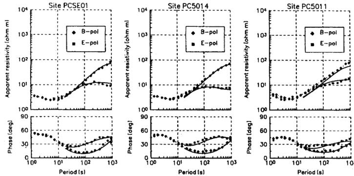
Fig. 4. Interpolated measured (dots) and modelled (line) apparent resistivity and phase as functions of period for 3 stations.
