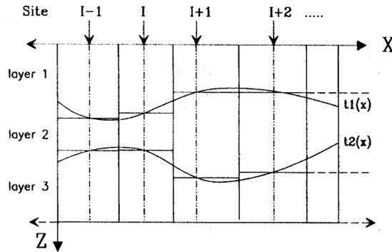
Fig. 1. 2-D model showing a juxtaposition of 1-D models with layer thicknesses described by polynomials  $t_1$  and  $t_2$ . Index  $I$  refers to station sites.
