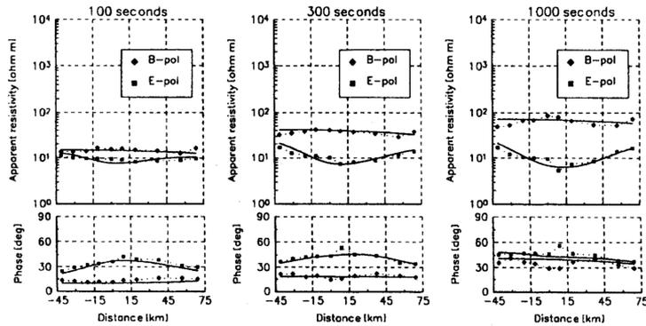
Fig. 3. Interpolated measured (dots) and modelled (line) apparent resistivity and phase as functions of the distance on the profile for 3 periods.
