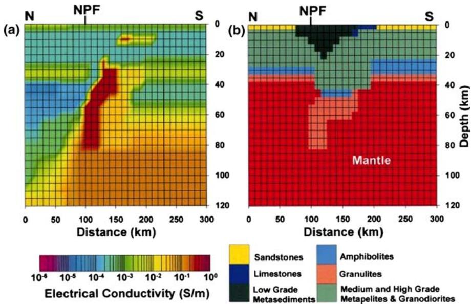
**Fig. 9** Conductivity model of Pyrenees (Pous et al. 1995b, c) and an associated model on structure and lithology used to integrate magnetotelluric data (model) with laboratory data on electrical conductivity of crustal and upper mantle rocks (Glover et al. 2000). Figure by courtesy of Elsevier
