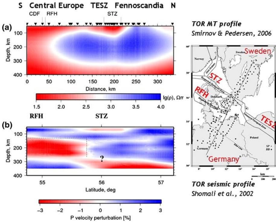
**Fig. 11** TOR-models along the TOR array region from North Germany via Denmark to southern Sweden (map to the left) crossing the Trans-European Suture Zone (TESZ). 2D resistivity model at top is from Smirnov and Pedersen (2006, 2007). Seismic P-wave model at bottom is from Shomali et al. (2002). RFH = Rinköping Fyn High, STZ = Sorgenfrei-Törnquist Zone. Figure by courtesy of Blackwell Publishing Ltd. and Maxim Smirnov
