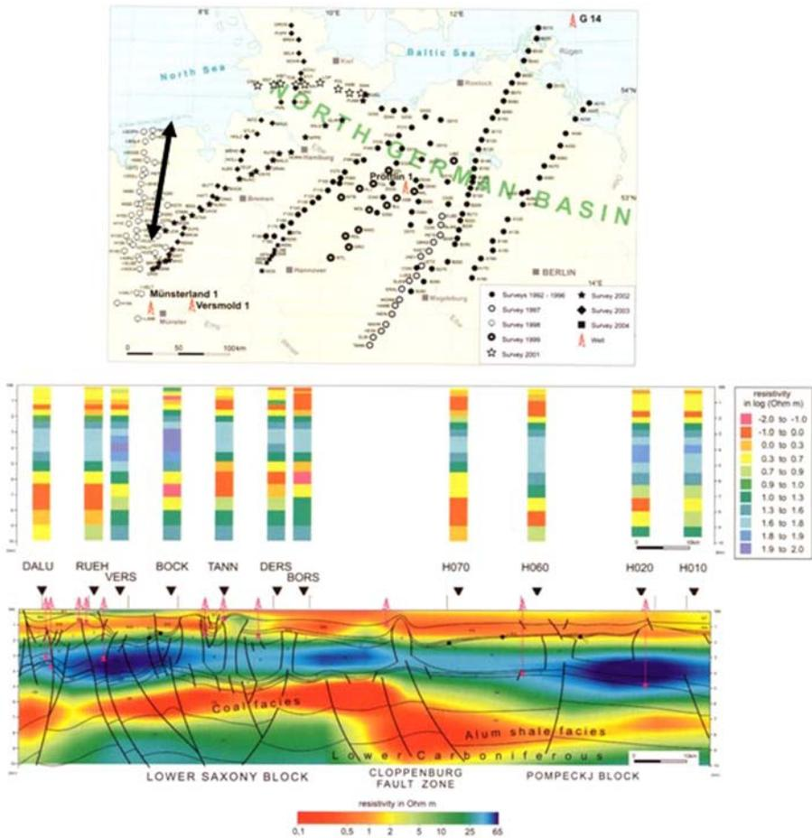
**Fig. 12** Magnetotelluric sites in North German Basin (top) and an interpretation superimposed on 2D resistivity model along the profile shown by double arrow in map (roughly NS-directed westernmost profile). Figure from Hoffman et al. (2005) (by courtesy from <http://www.schweizerbart.de>)
