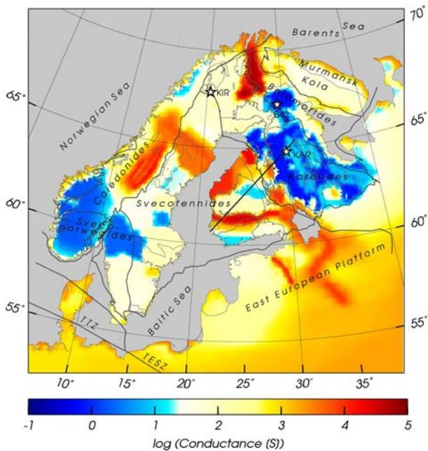
**Fig. 14** Crustal conductance (Smap) of Fennoscandia at the depth interval 0–60 km. Note that conductance of water areas is removed from the map. Figure from Korja et al. (2002). Figure by courtesy of Terra Scientific Publishing Company
