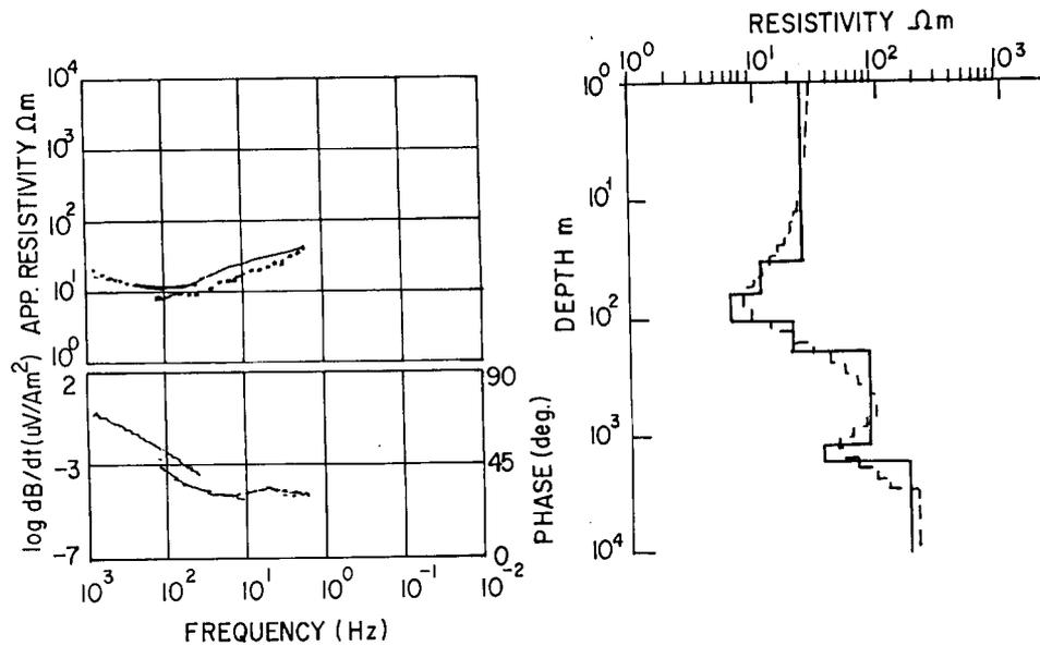
Figure 5. TEM and MT data from Ireland near a known sulphide deposit. The data have been subjected to joint inversion without static shift correction considering TEM data in the high frequency range (1000–50 Hz) and MT phase data. Good fit to phase data and misfit to MT apparent resistivity data can be seen. The two models shown on the right side of the figure are derived assuming initial half space (broken line) and sparsely parameterized model (solid line) (from Meju, 1996).
