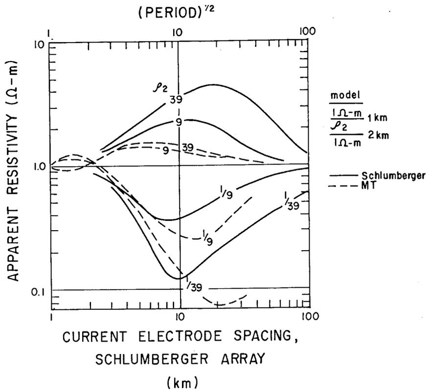
Figure 3. Comparison of the responses of the DC resistivity and MT methods for a 3-layer model. The responses for a resistive and conductive middle layer are different for both methods. MT apparent resistivity curve is more sensitive to a conductive layer than a resistive layer (from Vozoff and Jupp, 1975).
