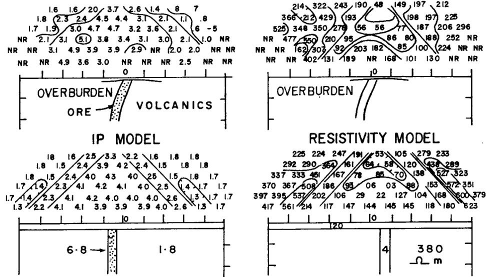
Figure 7. Observed (top) and computed (bottom) apparent polarizability and apparent resistivity data over the Flambean massive sulphide deposit, Wisconsin based on simultaneous inversion of IP (left) and resistivity (right) data sets (from Pelton et al., 1978).
