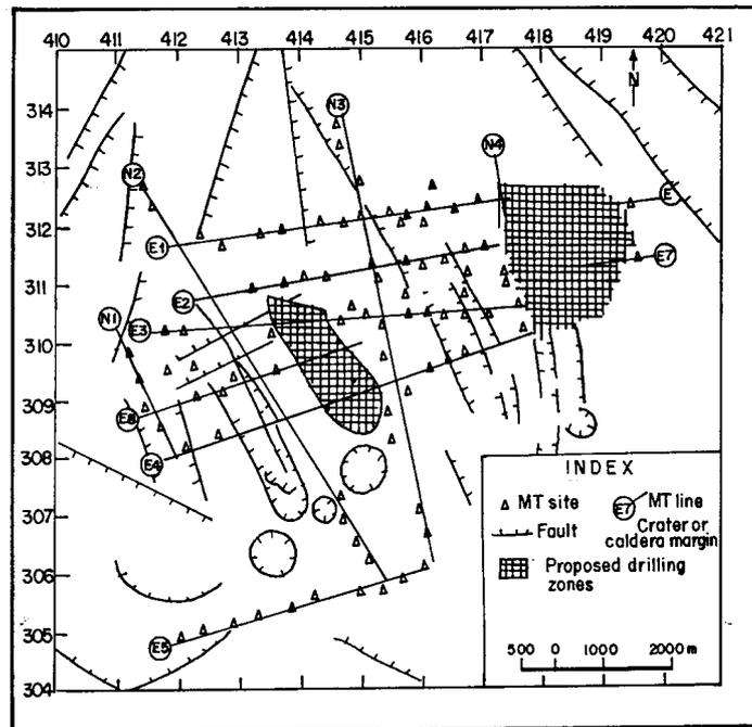
Figure 12. Proposed drilling zones for exploitable geothermal resources are shown by hatched lines, Chipilapa geothermal field, El Salvador. The inferences are drawn based on a combined interpretation of dipole-dipole resistivity and magnetotelluric data (from Romo et al., 1997).
