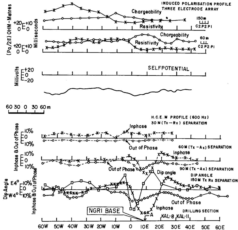
Figure 8. Various geophysical profiles – IP, SP, Resistivity, EM – near Aladahalli area, Karnataka, India. Mineralized zone (near 10E) is predicted from the integrated studies (from Jayaram, 1982, courtesy: G.S.I.).
