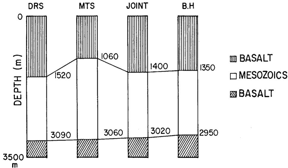
Figure 6. Models derived from deep resistivity sounding (DRS), MT (uncorrected) and from joint inversion of MT (corrected) and DRS data sets (Harinarayana et al., 1998). Results are compared with the deep borehole lithology.
