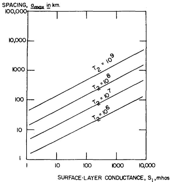
Fig. 2. The spacing for which the maximum apparent resistivity is recorded for a three-layer sequence with the middle layer being highly resistive.
