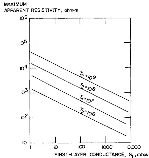
Fig. 3. The maximum apparent resistivity which is observed over a three-layer sequence with the middle layer being highly resistive.
