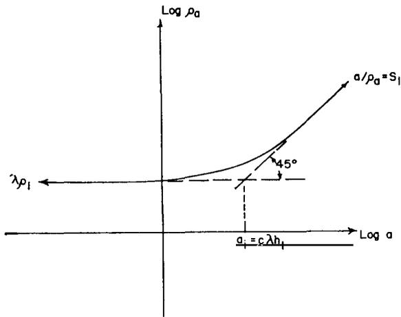
Fig. 1. The asymptotes of a two-layer dc resistivity sounding curve in which the second layer is highly resistive.
