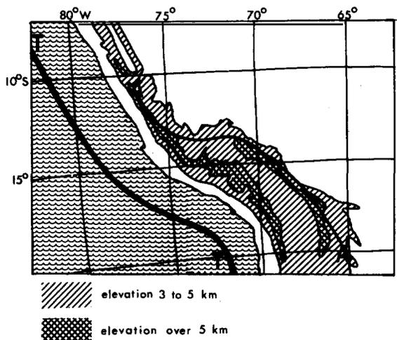
Fig. 1. Location of the conductivity anomaly of the Peruvian Andes.  $A-A$  = centre of conductive body after Schmucker et al. (1967).  $T-T$  = axis of Peru-Chile Trench.
