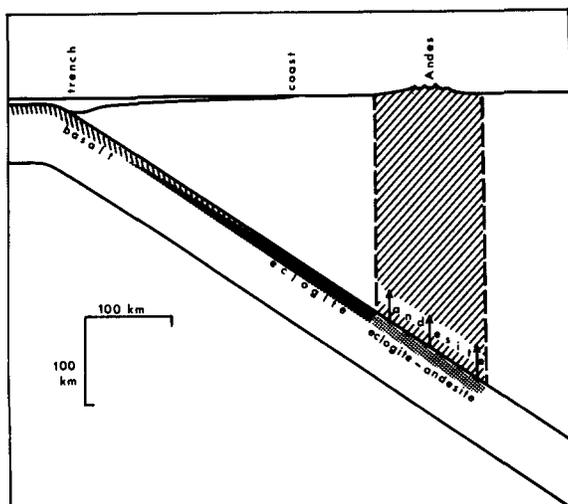
Fig. 2. A model based on the basalt–eclogite–andesite sequence of Ringwood and Green, which accounts for heating under the mountains by ascent of andesite in the shaded column. This column has reduced density through the andesite contamination, and accounts for dynamic uplift of the mountains.
