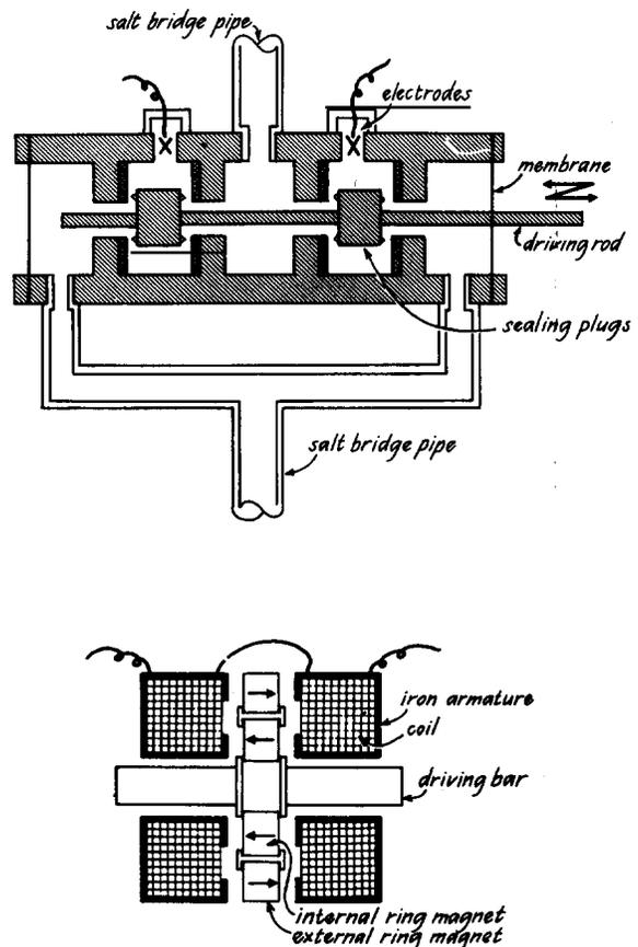
Fig. 17. Top: double pole double throw "water chopper". Bottom: low power driver for above
