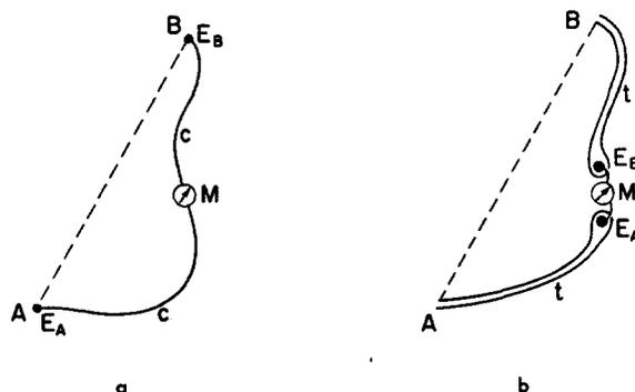
Fig. 8. a. Schematic representation of a cable-type electric field sensor and b. salt bridge version of the same instrument.  $E_A, E_B$  = electrodes,  $C$  = cables,  $t$  = salt bridge tubes,  $M$  = meter.
