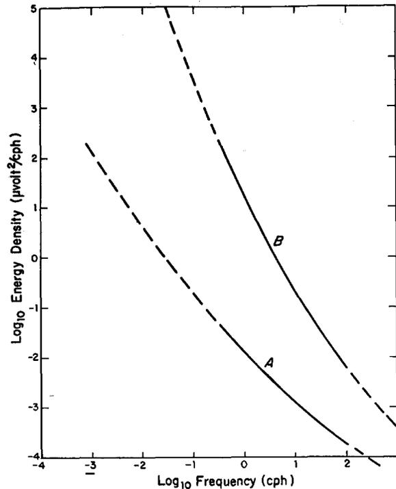
Fig. 15. Energy spectra of electrodes near the ocean floor. A for low noise electrodes, B for marginal electrodes.
