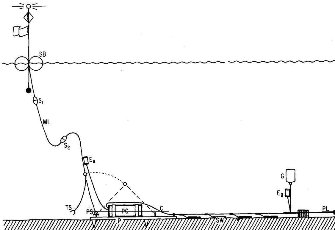
Fig. 10. Fixed electric field recorder on the sea floor. PC = recording voltmeter in pressure case; C = cable;  $E_A$  and  $E_B$  = electrodes; G = gasoline float; ML = mooring line;  $S_1$ ,  $S_2$  = swivels; SB = surface buoy; PL = pulling wire; SW = sash weights; P = platform; PS = permanent shackle; TS = temporary shackle.
