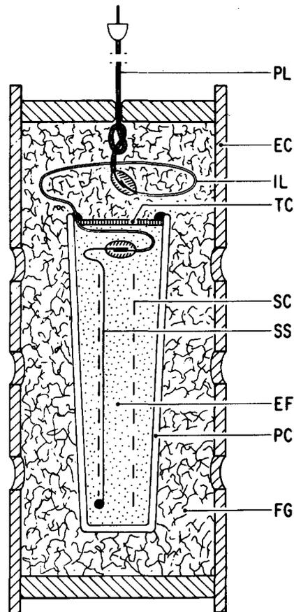
Fig. 13. Silver–silver chloride electrode cross-section.  $PC$  = porous container;  $SC$  = silver gauge cylinder;  $SS$  = silver stem;  $EF$  = electrode filler (silver chloride);  $TC$  = top cap;  $EC$  = electrode housing;  $FG$  = shock absorber (pyrex wool);  $PL$  = plug;  $IL$  = intermediate lead.
