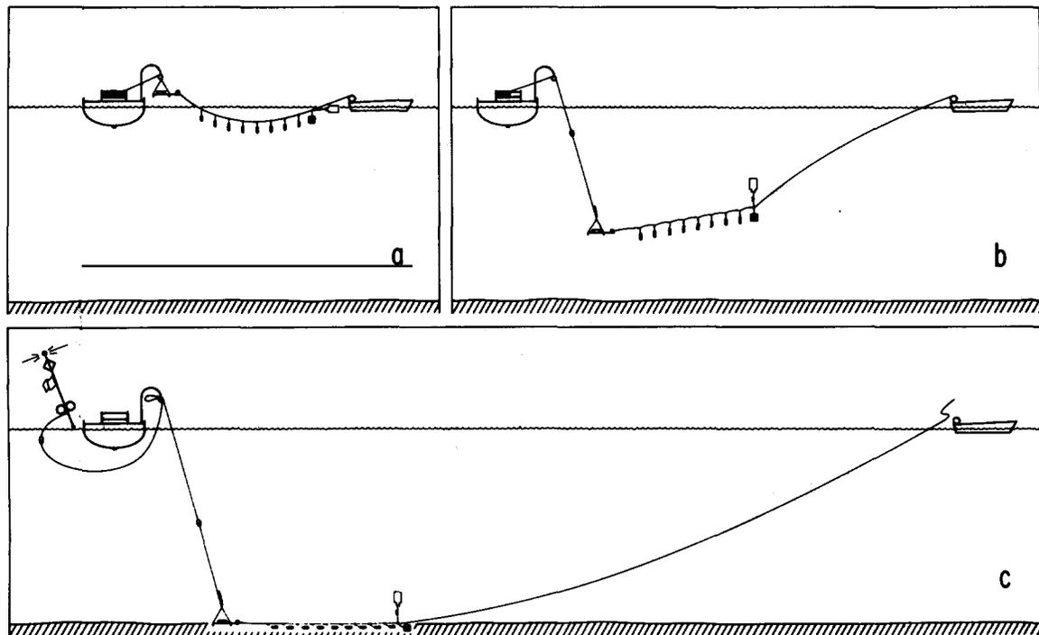
Fig. 11. Installation of long cable electric field recorder on the sea floor. a. The cable is stretched at the surface and ballasted to create a 0.5 m/sec natural sinking speed. b. Lowering from ship at 0.5 m/sec and stretching from small boat by means of long pulling wire. c. Release of pulling wire and launching of float.
