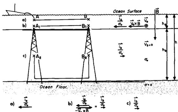
Fig. 9. Response of GEK and fixed electrodes in a simple two-layer flow. The surface layer of thickness  $h_a$  moves with velocity  $V_a$ , cutting vertical magnetic component  $B$  to produce motional field  $V_a \times B$ . Electric currents with density  $i_a$  set in surface layer return in stationary lower layer (density  $i_b$ ). Layer thickness  $h_a$  (above) and  $h_b$  (below). a. Response of GEK; b and c. Response of fixed electrodes in moving and stationary layers, respectively.
