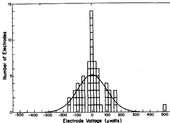
Fig. 14. Electrode voltage distribution of 66 Ag-Ag Cl electrodes. Gaussian distribution with same area and same standard deviation also shown.
