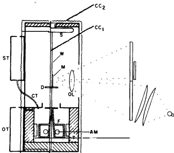
Fig. 7. Automatic orientation of magnetic suspension in sea-floor magnetometer. At launching magnets  $AM$  in float  $F$  rest in tank  $T$ . Oil dripping through capillary tube  $CT$  from storage tank  $ST$  fills tank  $T$ . Float  $F$  rises and connects with discs  $D$  and mirror  $M$ . Subsequent mirror rotations are picked up by grid-type optical lever.  $CC_1$  and  $CC_2$  = calibration coils;  $OL$  = objective lens;  $OT$  = oil overflow tank.
