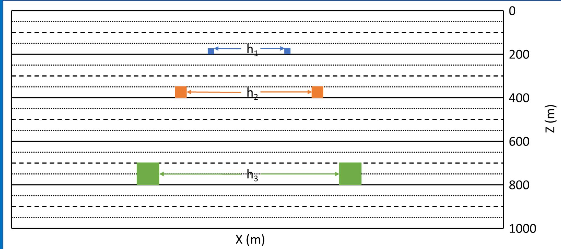
Three model cases for resolution evaluation between standard TEM data and ITEM processing results using **elongated conductors**. Conductor length in each case is 1000 m. The distance,  $h$ , between the pair of bodies is varied (increment = 25 m) to determine the minimum distance where two signals can be observed in the data.
