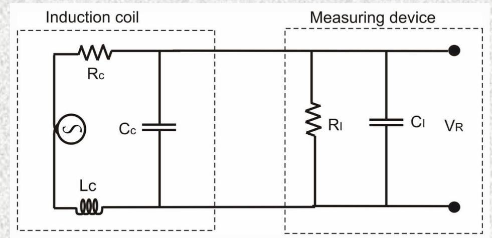
Equivalent electrical circuit to an induction coil sensor.
