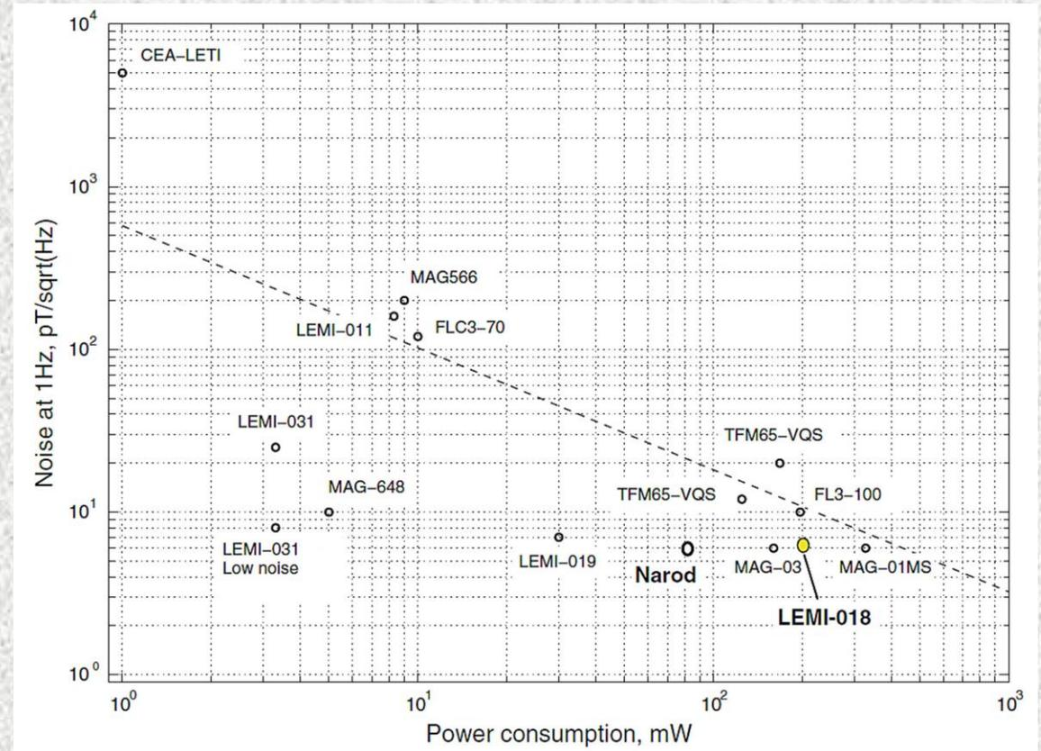
Fluxgate power consumption versus noise level (Korepanov & Marusenkov, 2012)
