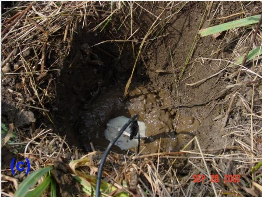
Installed porous pot electrode
