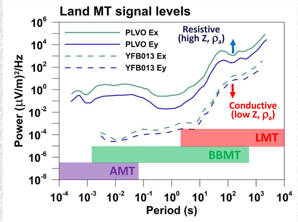
Power spectra of MT signal levels. Land data are from a relatively resistive region in central Canada (PLVO) and a relatively conductive site in southwestern Australia (YFB013).
