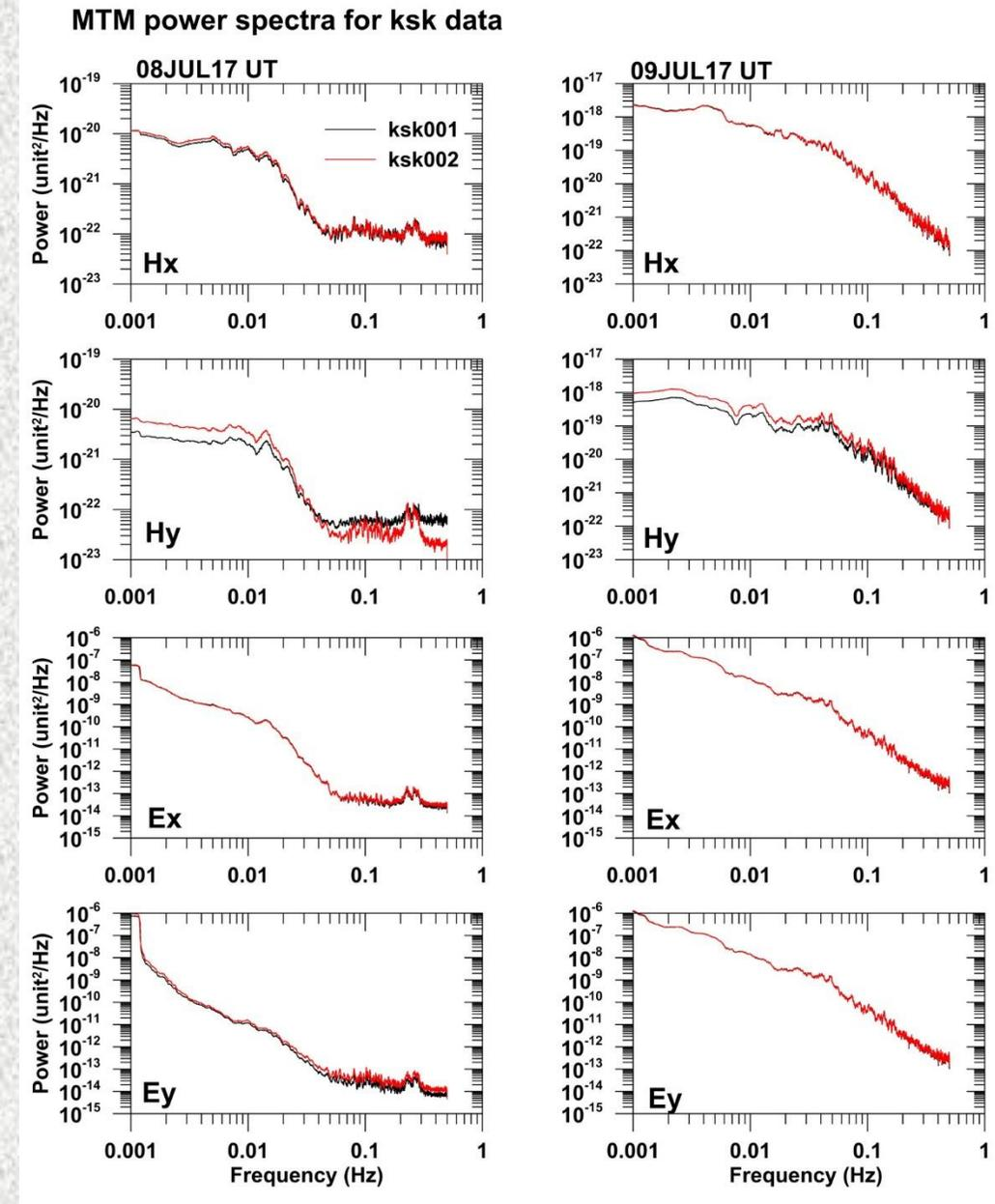
Examples of spectra during extremely low signal levels showing recording system limits.
