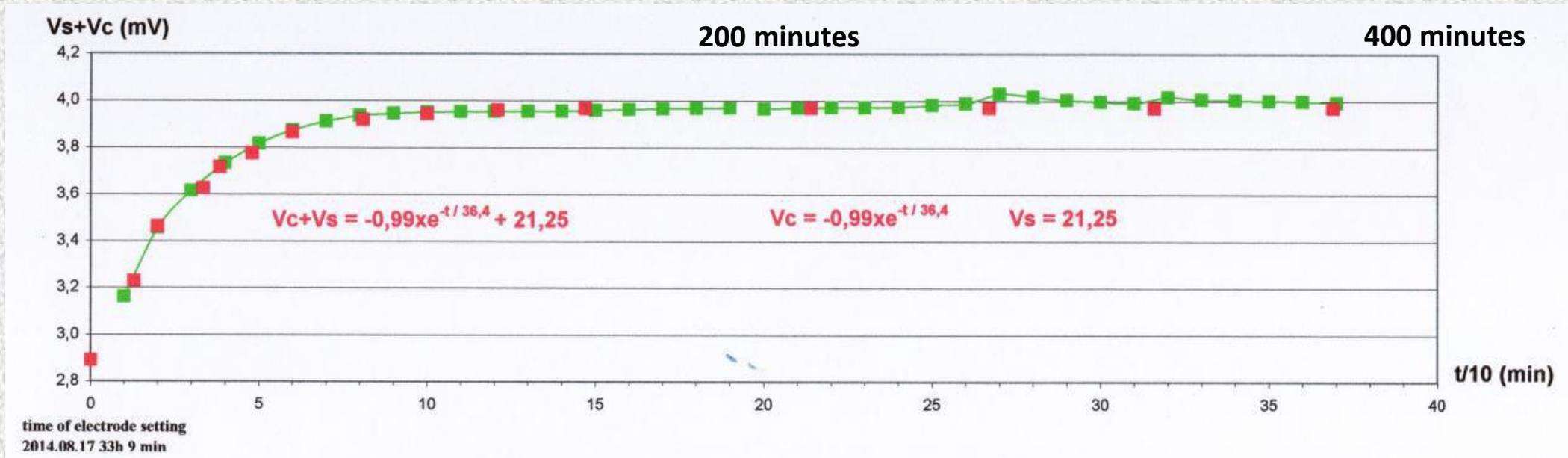
An example of the observed decay of a contact potential (S. Andras, "Results of test measurements")
