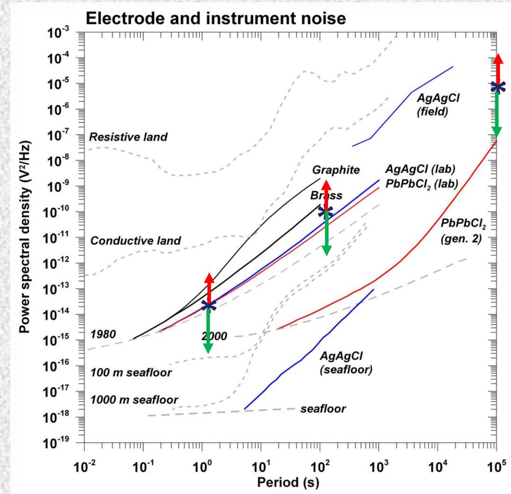
Comparison of noise levels of electrodes and telluric recording instrumentation with signal levels. Signal levels are for 100 m long dipoles.
