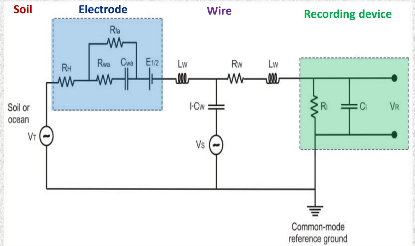
Circuit representation of a telluric measurement (modified from Zonge & Hughes 1985).
