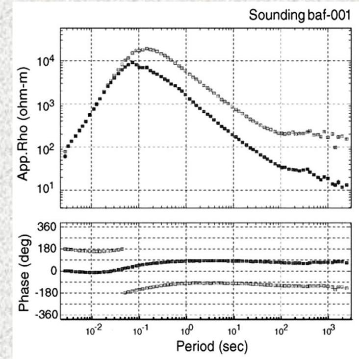
MT response from Baffin Island, northern Canada (Evans et al. 2003). Solid symbols are the xy- and open symbols are yx-component. Response at  $<0.1$  s are affected by high contact resistance causing the earth-electrode-recording system to act as an low-pass filter.
