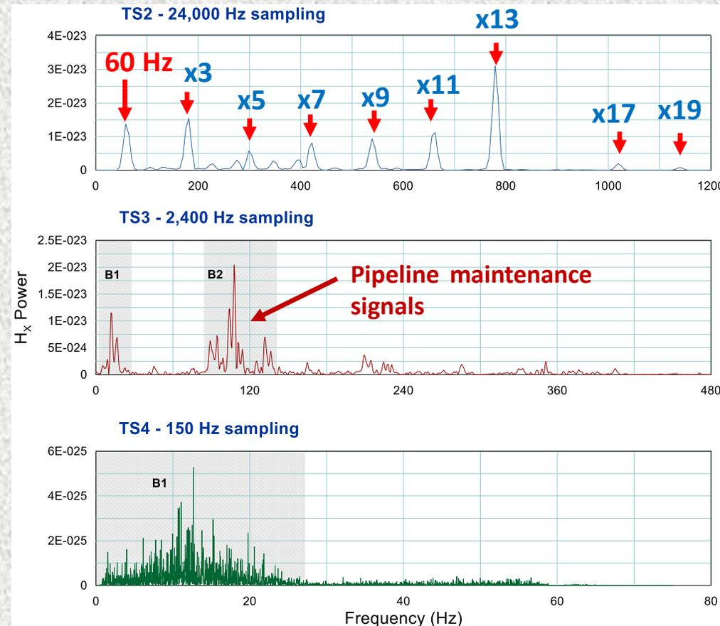
$H_x$  spectra for each of three MT data sampling frequencies recorded on November 10, 2014 at site aqi08 near the Boundary Dam Power station, Saskatchewan (McLeod, 2016).
