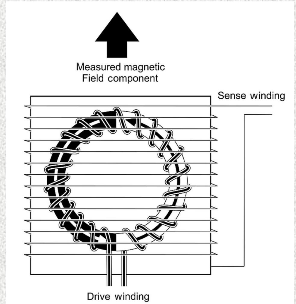
Ring-core fluxgate sensor (Miles et al., 2017)
