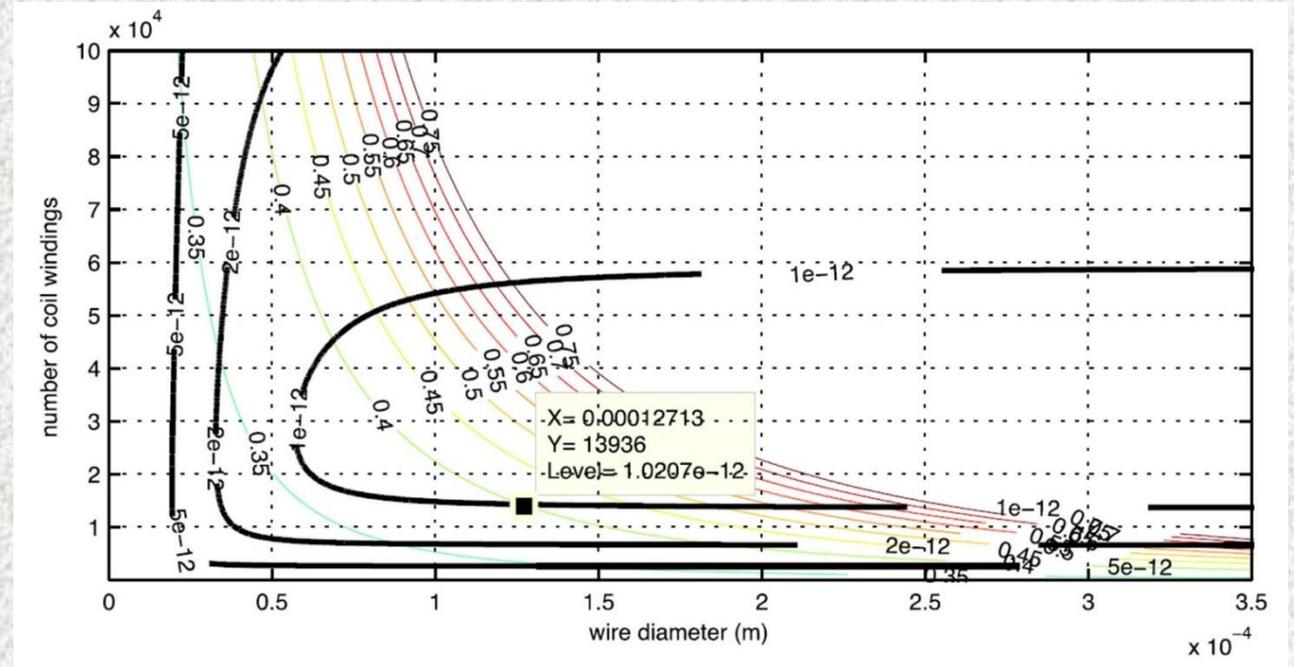
Optimizing mass and noise levels of coil (Hamad & Macnae, 2014) showing noise level in T at 1 s in black and coil mass in kg in colour.
