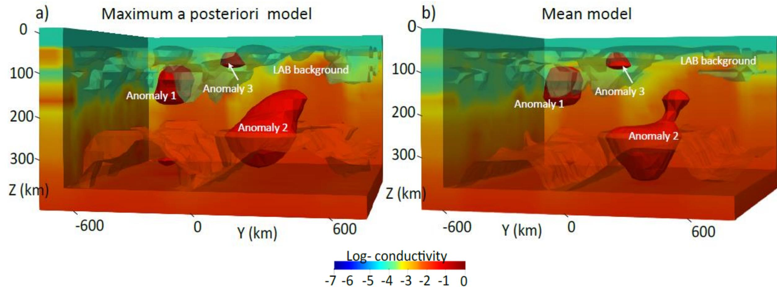
Joint probabilistic inversion of 3D MT and SW synthetic data
